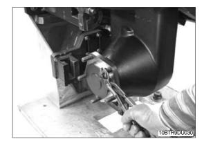
④ Disengage snap ring from the annular groove on the housing.
