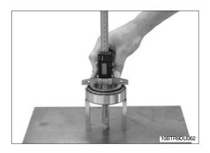
(5) Insert adjusting washer into the bearing hole and force in bearing outer ring until contact is obtained.
