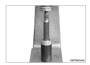
(4) Remove spur gear from the housing.
