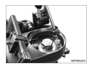
② Grease the O-ring and install it into the annular groove on the cover (see arrow).
