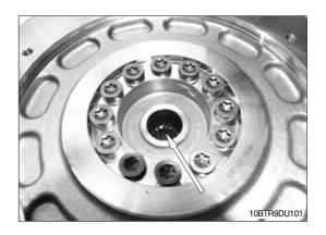
⑤ Apply grease evenly on the shaft at the electric motor.
