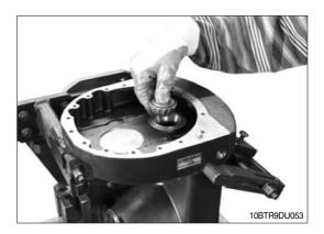
6 Wet inner gearing at the spur gear evenly with Loctite 270.
