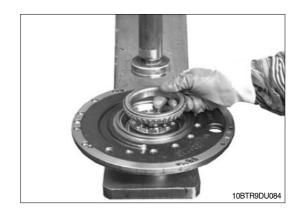
Adjust rolling torque of the connection plate bearing (fig. 085~097).
