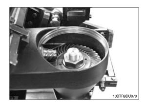
Six and support the locking device (S) on the gear shaft.
