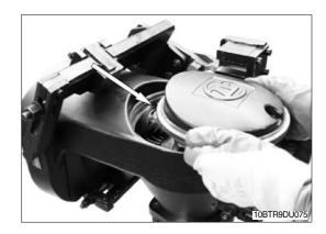
② Insert snap ring into the annular groove on the housing and fix the cover.
