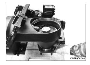
② Support unit on the gear shaft. Use a press to bring crown wheel and suitable sleeve to contact position.
