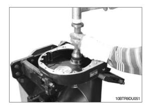
④ Press-on the bearing inner ring until contact with the bevel gear shaft is obtained.
