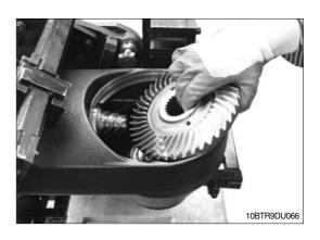
Press on the bearing inner ring until contact with the gear shaft is obtained.
