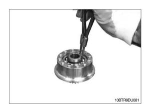
⑤ Press bearing inner ring onto the bushing as illustrated.
