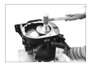
③ Support the bearing inner ring with a suitable sleeve and press it off the bevel gear shaft.
