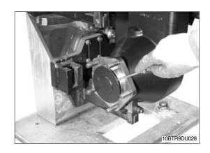
② Install locking device (S) on the gear shaft (see arrow) thus blocking the gear shaft against rotation. Loosen both hexagon nuts on the bevel gear shaft one after the other.
