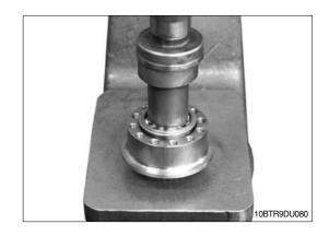
⑤ Fix ball bearing on the input pinion by means of a retaining ring.
