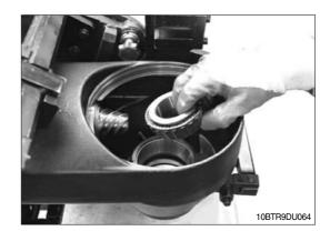
Wet inner gearing at the crown wheel evenly with Loctite 270.
